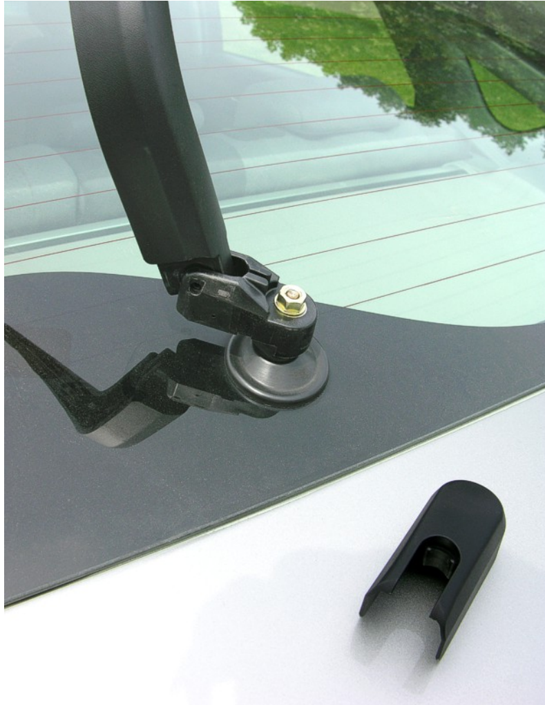
Rear Hatch Wiper (Toyota Part: 85124 - 44140)
